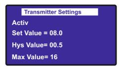
**Set Value :** Diesel engine stop set pressure value.
