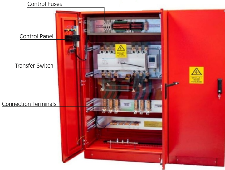
Figure-34: TRF.OT Panel Inside View
